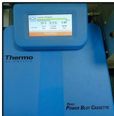
Figure 16: Power blot cassette for semi-dry transfer
