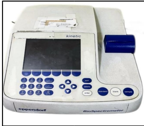
Figure 11: Bio-spectrometer used for RNA quantification.
