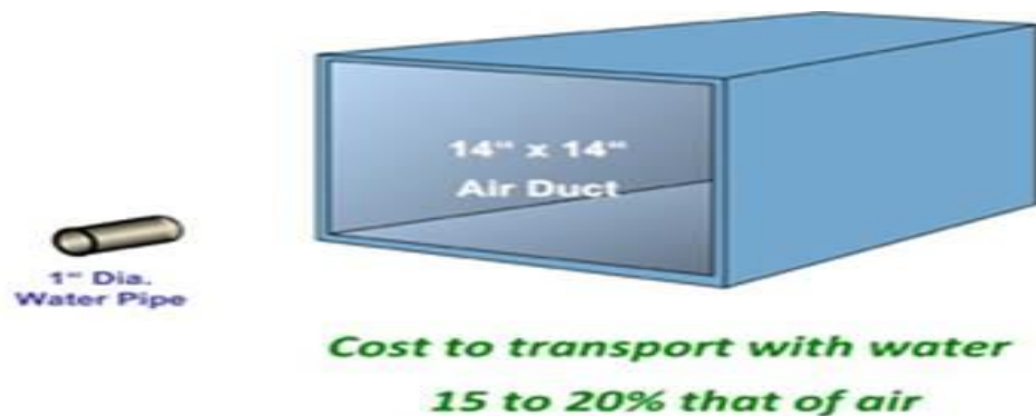
Figure 6:- Air versus Water Duct in chilled beam
