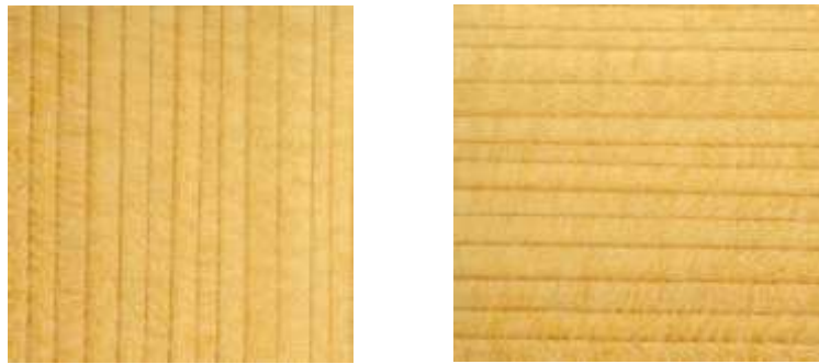
Fig.8 Fiber orientation in relation to properly positioned cores (left), and improperly positioned cores (right) in core mounts.
