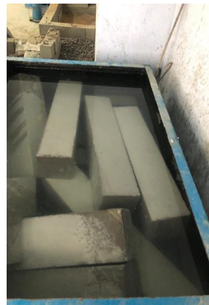
Fig 4.4 Curing of beams
