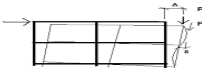
Fig.1.2: Illustrates the P-Delta effect in the framed structure [6]
