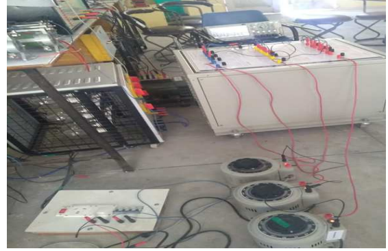
Fig. 10: Setup of the three- to-five phase transformer developed in lab.
