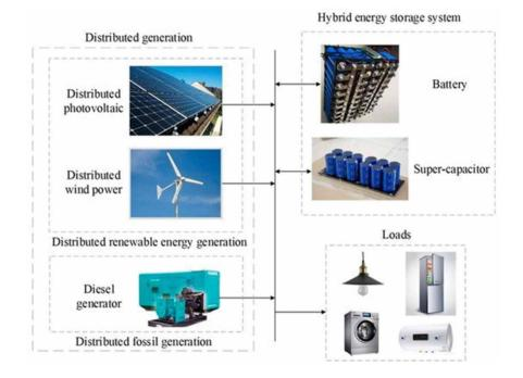
Figure 7. Hybrid Energy storage system with distributed power system (Liu et al., 2018).
