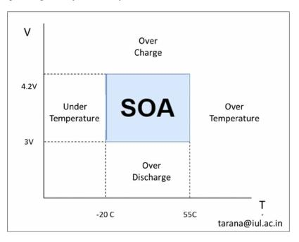
Figure 15. Temperature range for charging/discharging of battery.
