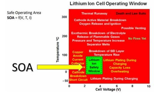
Performance of battery is an important parameter in a battery management system (BMS). The battery protection management involves two specifics protection parameters i.e. electrical and thermal protection. The electrical protection helps the battery from getting damage i.e. its use outside the surface operating area, while the thermal protection helps to control the passive/active temperature and maintain its surface of operating area.
