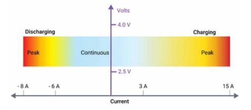
Figure 13. Current-Voltage range of lithium-ion cells.
