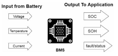
Monitoring and control are applied to all individual cells known as modules. Lithium-ion batteries are rechargeable having maximum energy density. These batteries are considered as standard choice for many appliances such as laptop, mobiles, electric vehicles etc. Their operations are in safe mode but it is critical during charging and discharging mode. If the voltage and current of any battery goes beyond
